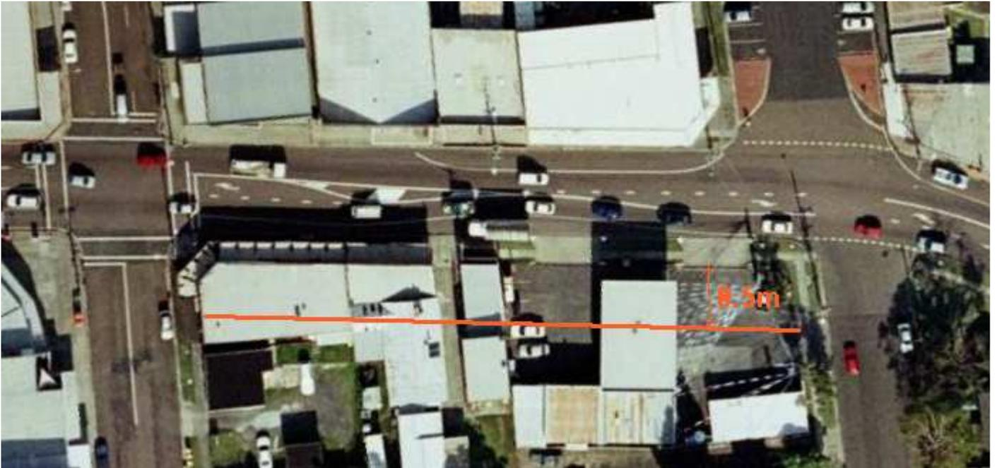
The whole carriageway will require reconstruction from kerb to kerb. One advantage of the widening will allow sufficient width to stage the construction without closing down one carriageway completely.
